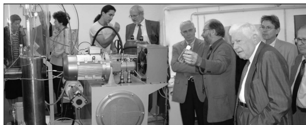
Figure 2. Pilot plant for high-pressure treatment of foodstuffs (TU Berlin).
